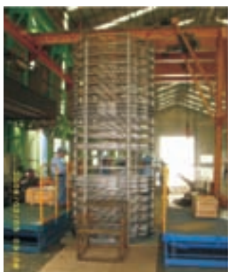
▲ Fabrication of test TSC---basket assembly
