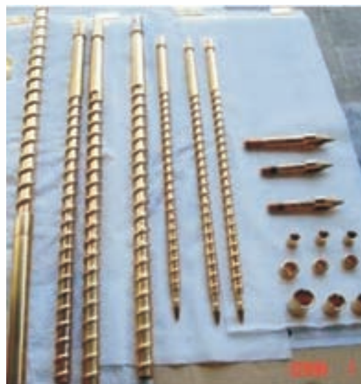
▲ Fig. 2. Photo of large plastic screws coated with TiN film
