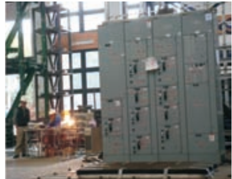
▲ Motor Control Center Seismic Qualification
