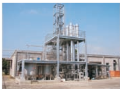
▲ Ethanol Distillation and Dehydration System
