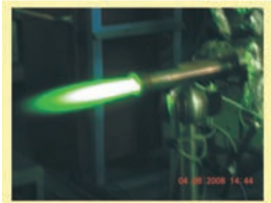
▲ Fig. 1. Photo of novel steam plasma torch in operation
