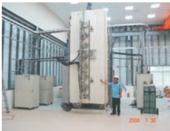
▲ Fig. 1. Photos of plasma coating system with a huge vertical chamber (1300 H 3900 mm), located at Gong-Sung Industry Park
