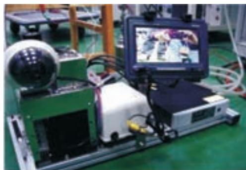
▲ The 75 W surveillant system was driven by hydrogen storage tank filled with Pt/AC.
