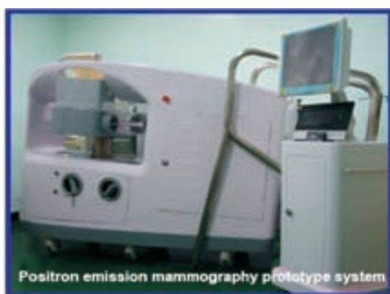
▲ Positron emission mammography prototype system and its breast phantom image (F-18-FDG, without any correction).
