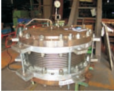
▲ Metal Expansion Joints Hydraulic Tests
