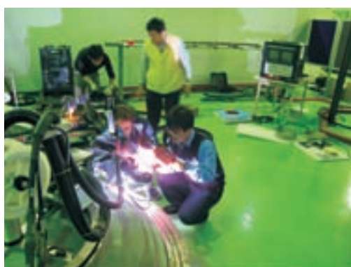
▲ Operation mock-up--- Closure welding
