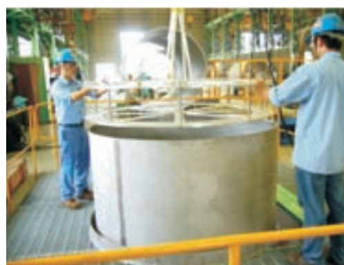
▲ Fabrication of test TSC---shell go gauge test
