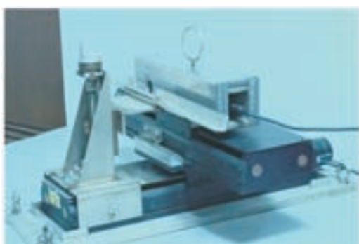
▲ Micro-visual inspection system in hotcell
