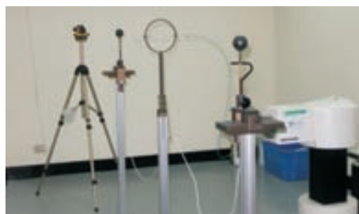
▲ Fig. 1. Brachytherapy source calibration standard system
