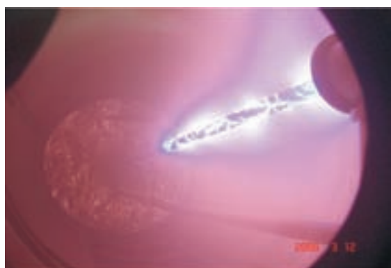
▲ Fig.3. Photo of arc-spots moving on the surface of cylindrical target during coating process
