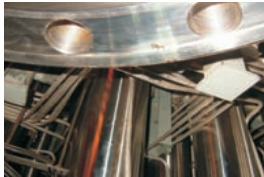
▲ Arc strike found on the surface of motor casing of reactor internal pump
