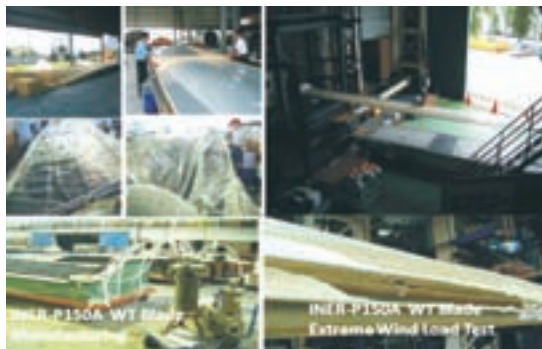
▲ The manufacturing process and the extreme load test of 150 kW WT blade
