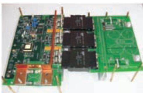
▲ A high-efficiency 5-kW SOFC Power Conditioning System with 97.1% peak efficiency
