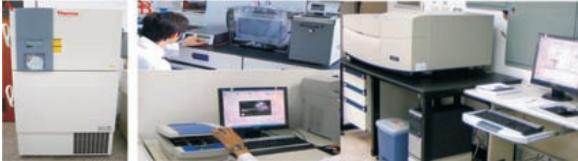
▲ (A) Sample freezer; (B) The instruments of Two-Dimension Difference Gel Electrophoresis (2D-DIGE), including 1D-IEF, 2D-SDS-PAGE and Typhoon Trio scanner.
