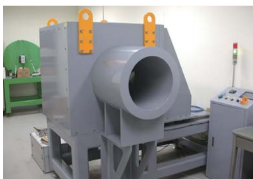
▲ Radiation Measurement Instrument Calibration Facility Capable of Lowering Scattered Radiation And Shielding Background Radiation
