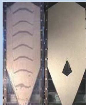
▲ Flow of Silica Sand in 2-D Hopper
