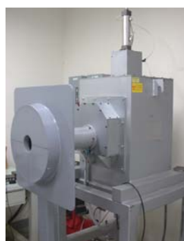
▲ Self-made ^{137}\text{Cs} Irradiator and Collimator
