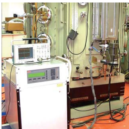
▲ High Power Pulsed Magnetron Sputtering Coating System
