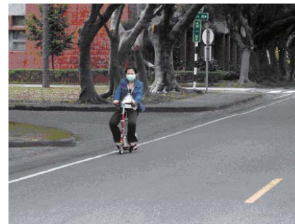
▲ A 120 W scooter Powered by a PEMFC with H 2 Fuel Supplied by a Hydrogen Tank of Pt/AC
