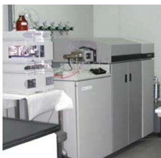
▲ Matrix Assisted Laser Desorption Ionization-quadrupole-time of Flight Mass Spectrometer (Maldi-QTOF MS)
