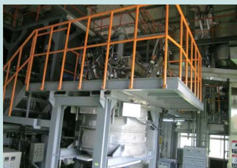
▲ A New Arc Melting and Fiber Blowing Device
