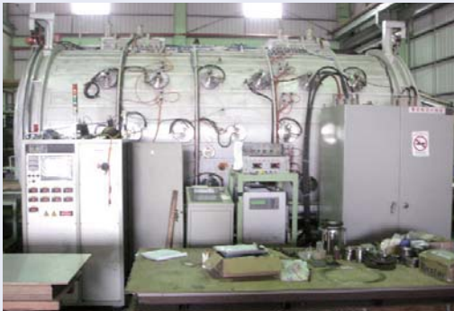
▲ Advanced Large Plasma Coating Integrated System
