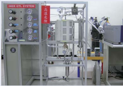
▲ High-pressure High-temperature DME Reaction System.
