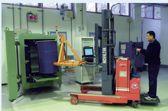
▲ Measurement on Gross Specific Activity of Scrap Metal for Release
