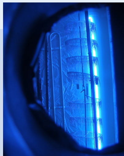
▲ The Plasma Coating Condition of HIPIMS System for Depositing the Needles by Cylindrical Target
