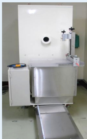
▲ Irradiating Apparatus with Attenuating Medium Using a Discarded Co-60 Source
