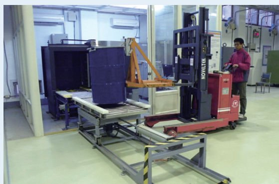
▲ Sampling of Releasing Scrap Metal for Verification of Specific Activity
