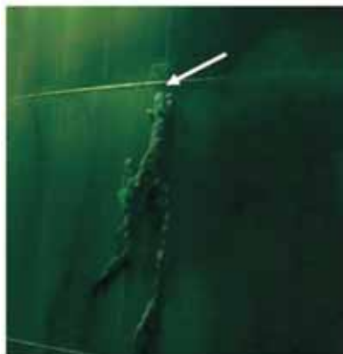
The visual test indicates the leakage around the fusion zone.
