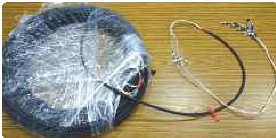
Fig. 12-core fiber optic cable and ST connector for testing
