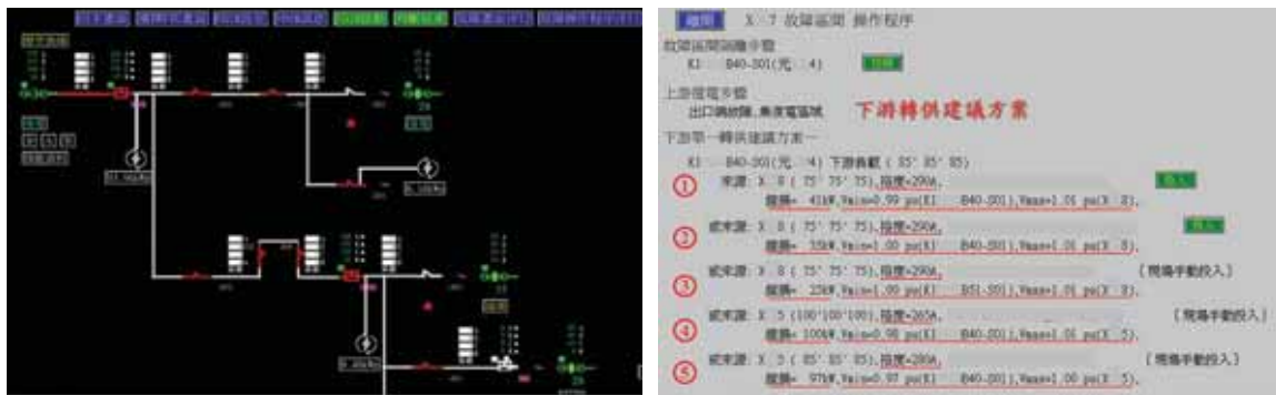
Figure 3. Integration of distribution power flow calculation program and feeders dispatching platform
