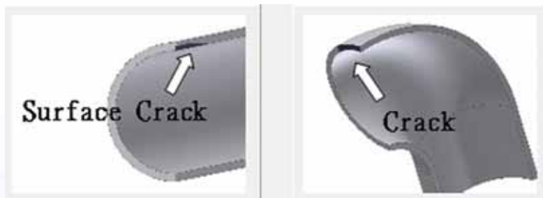
Fig. 1. Evaluation of cracks in piping components
