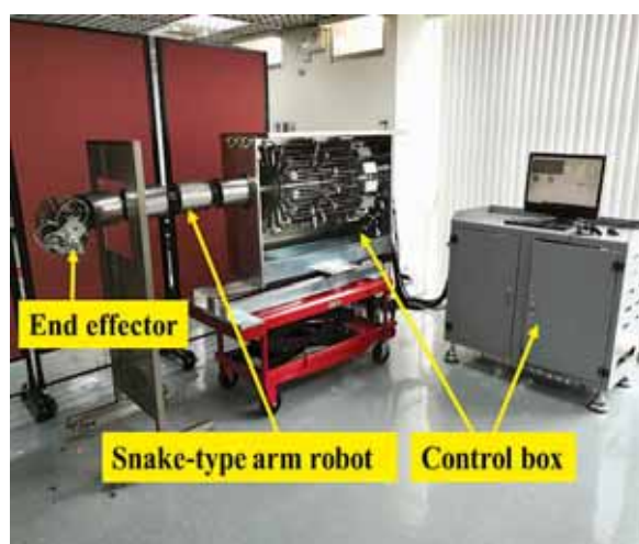
Fig.1. Remote control snake-type robotic arm
