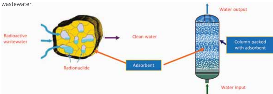
Fig.1. Working mechanism of inorganic ion-exchange adsorbent
