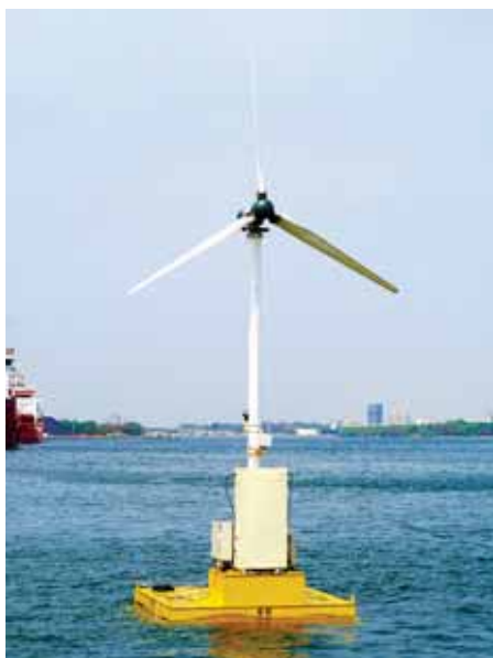
Fig.4. The field test of scaled floating wind turbine at Anping Port
