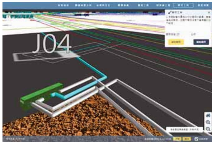
Fig.5. Presenting 3D profile of underground distribution feeders on commercial GIS
