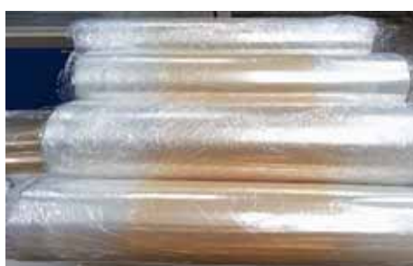
Fig. 1. Samples of roll-to-roll GPE membrane
