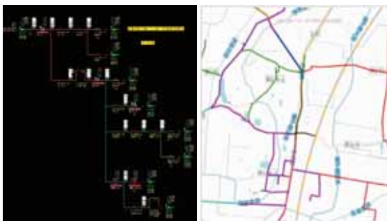
Fig.2. After SCADA (left) finishes FDIR process, GIS (right) visualizes the feeder operation status on the map.
