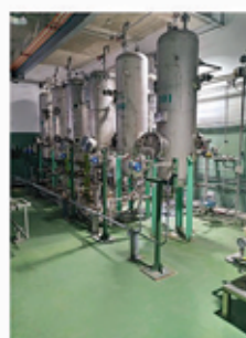
On-site adsorption equipment for washing waste liquid
