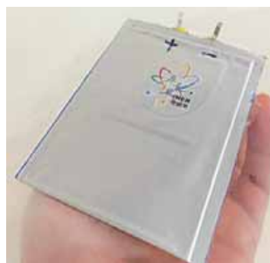
Fig. 3. Left: Charge and discharge curves of the aluminum plastic film battery. Right: A GPE LIB sample.
