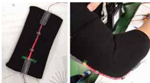
Fig.3. Elastic waveguide integrated with elbow pads
