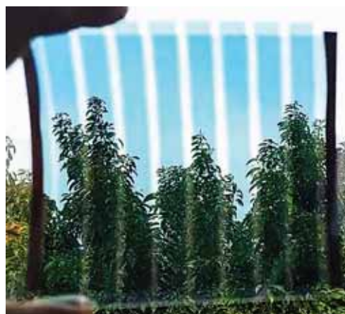
Fig.2. Flexible transparent organic solar cell modules developed by INER
