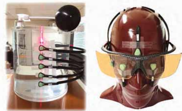
Fig.5. Characteristic study on the effect towards irradiation results with different dosimeter intervals and using lead glasses.
