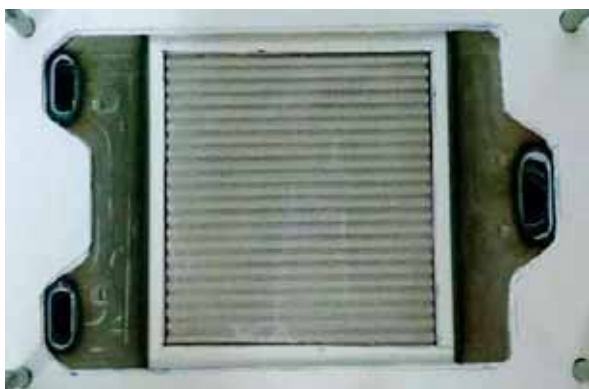
Fig.5. Glass-ceramic sealing strips as stack sealant
