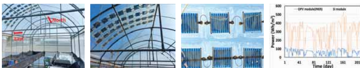
Fig.2. (a) Tunnel greenhouse with one end toward north direction, (b) All modules mounted on the curved roof, (c) Serially-connected modules via metal fasteners as terminal contact for each panel, and (d) Daily energy output per active area of OPV and Si-PV panels.
