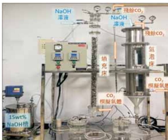
Fig.1. Bench-scale CO 2 carbonation test unit
