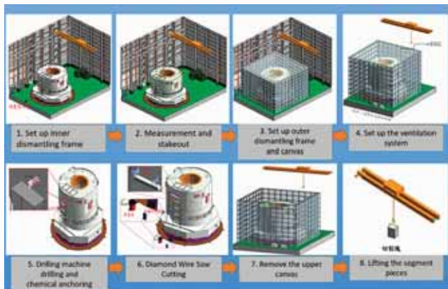
Fig.2. Biological Shield Dismantling Method
