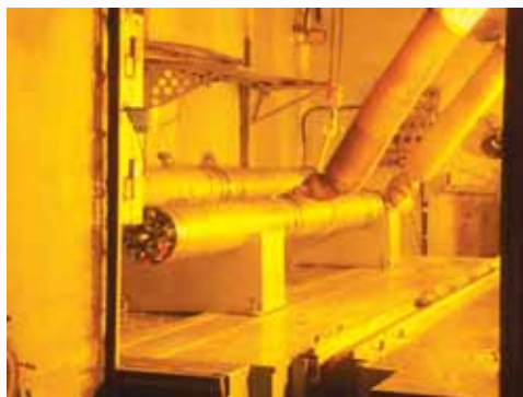
Special design storage casks installed in Hotcell
