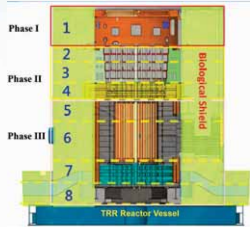
Fig.1. Phases of Biological Shield Dismantling Project
