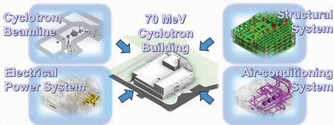
Integration of Cyclotron and Building Systems Interfaces Using BIM Technology
