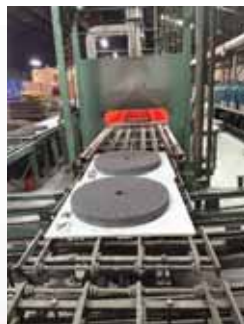
Desiccant Wheel sintering
