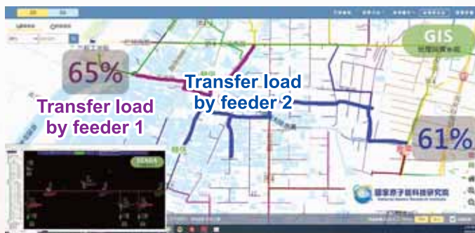
(b) Multi-segment load transfer An example of multi-segment load transfer
