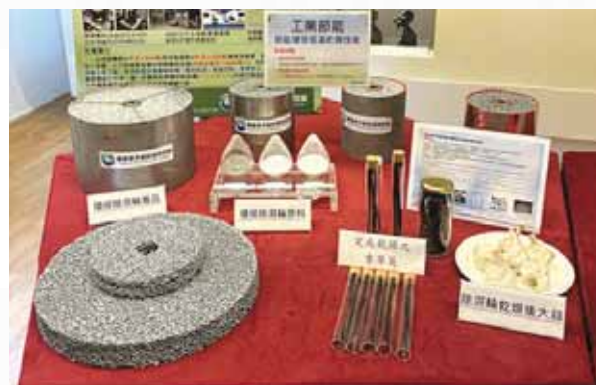
Desiccant wheel made from aluminum waste
