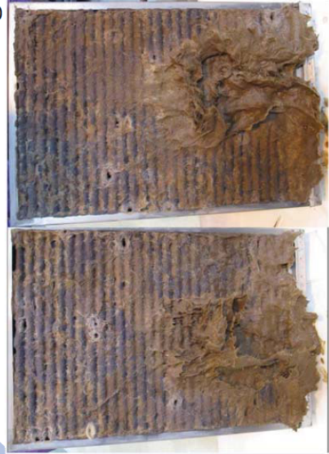
Figure C-8 MNPP-CET01 Debris Bed after Fin Removal
