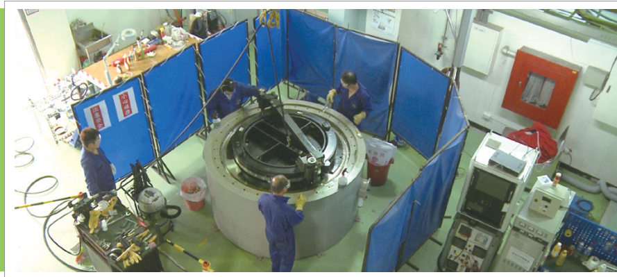
▲ Fig.4 Dry Run for TSC Top Lid Removal.
