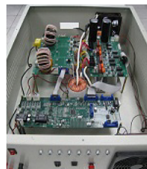
▲ Fig.6 5 kW bidirectional power converter with high efficiency and seamless control
