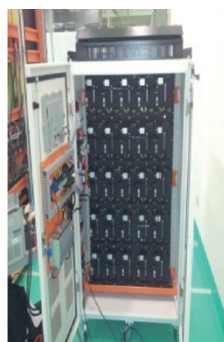
▲ Fig.4 Three phase 15 kW AC/DC bidirectional real and reactive power converter
