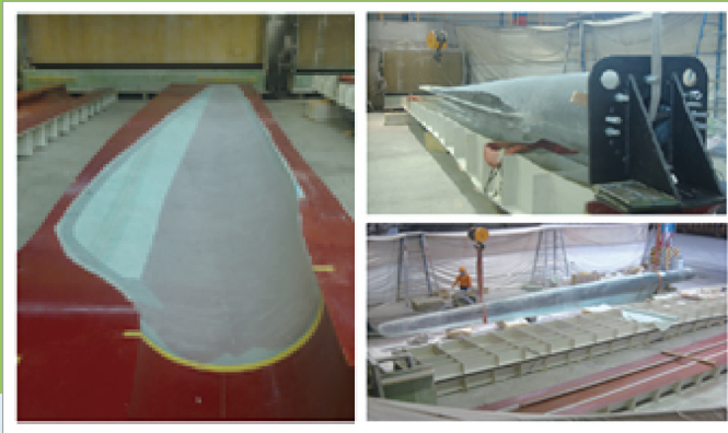
▲ Fig.10 Manufacture and test of the 2 nd -generation wind turbine blade.
