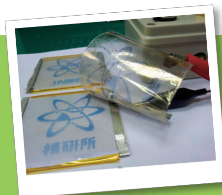
▲ Fig.5 150cmx90cm flexible solar cell building module (left) and 10cmx10cm flexible patterned energy-saving electro chromic window module (right).
