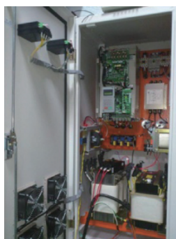
▲ Fig.4 Three phase 15 kW AC/DC bidirectional real and reactive power converter
