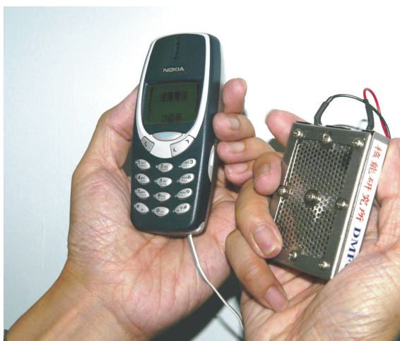
▲DMFC Power Pack 350 mW (25°C, 3wt.% MeOH)
