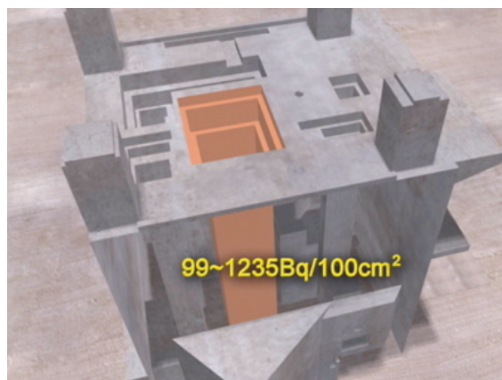
▲濕貯槽拆除3D模擬
