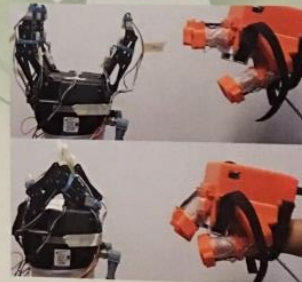
The fingers on the haptic glove directly control the gripper on a robotic arm, enabling natural grasping.
