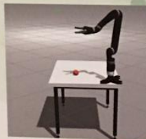
In this first stage of simulation, the mounted arm can interact with objects like the red ball shown
