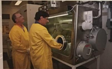
Workers sort through exhumed waste in a glovebox at the Idaho Site's Pit 9
