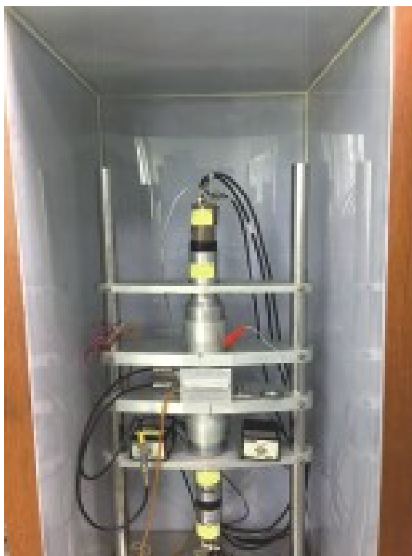
Fig. 3 4\pi\beta-\gamma measurement system
